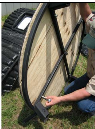
1. Loosen the four floor bolts with 9/16" socket wrench.
